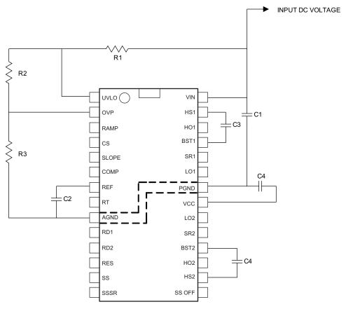
Figure 35. Layout of Components Around VIN, VCC, AGND, PGND UVLO, OVP, REF, BST1, BST2, HS1, and HS2
