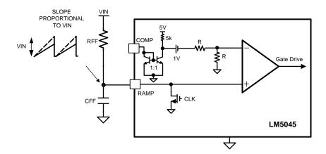
Figure 17. Feed-Forward Voltage Mode Configuration
