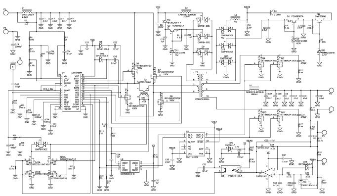
Figure 19. Evaluation Board Schematic
