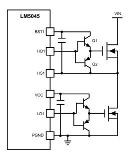
Figure 31. Bipolar Totem Pole Arrangement
