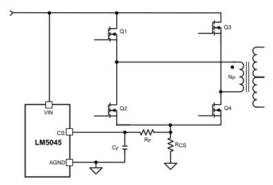
Figure 28. Resistor Current Sense
