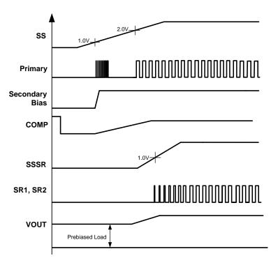
Figure 15. Prebias Voltage Start-up Waveforms
