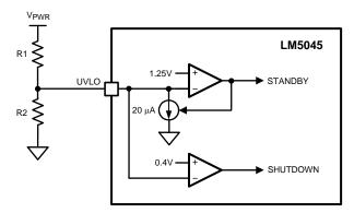
Figure 22. Basic UVLO Configuration
