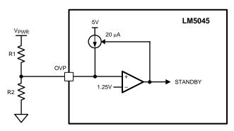
Figure 23. Basic OVP Configuration
