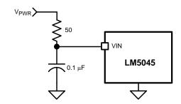
Figure 20. Input Transient Protection
