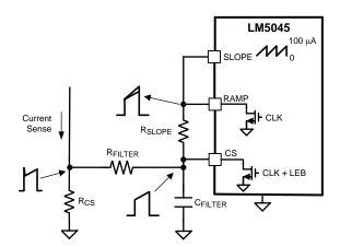
Figure 18. Current Mode Configuration
