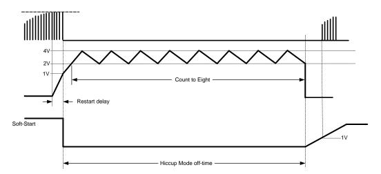
Figure 29. Hiccup Mode Delay and Soft-Start Timing Diagram
