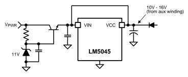
Figure 21. Start-Up Regulator For  $V_{PWR} > 100 \text{ V}$
