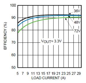
Figure 33. Application Board Efficiency
