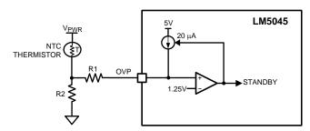
Figure 26. Remote Thermal Protection
