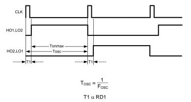
Figure 12. Timing Diagram Illustrating the Maximum Duty Cycle and Dead-Time Set by RD1
