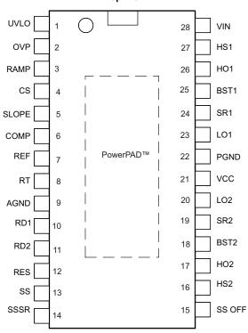
RSG Package 28-Pin WQFN, 5 mm × 5 mm Top View
