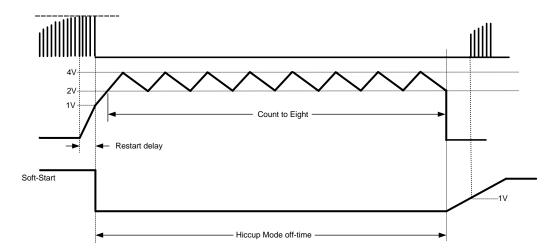
Figure 10. Hiccup Mode Delay and Soft-Start Timing Diagram
