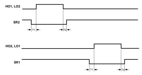
Figure 13. Synchronous Rectifier Timing Diagram
