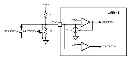
Figure 25. Remote Standby and Disable Control
