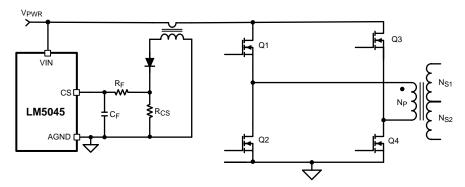
Figure 27. Transformer Current Sense
