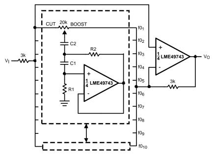
Figure 44. 10 Band Graphic Equalizer
