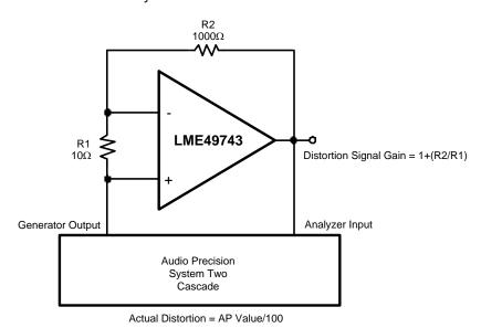
Figure 33. THD+N and IMD Distortion Test Circuit
