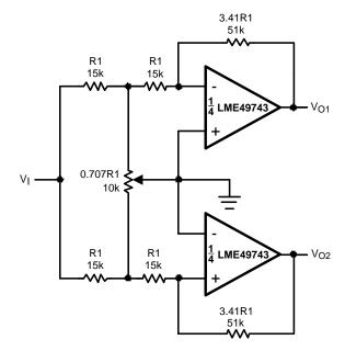
Figure 39. 2 Channel Panning Circuit (Pan Pot)
