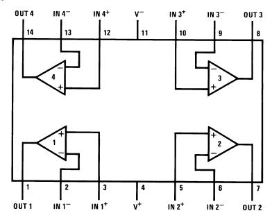
Figure 1. TSSOP Package See Package Number PW0014A
