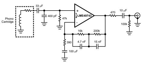
$A_{\nu}=35~\text{dB}$   $E_{n}=0.33~\mu\text{V}$  S/N = 90 dB f=1~kHz A Weighted,  $V_{\text{IN}}=10~\text{mV}$  at f=1~kHz
