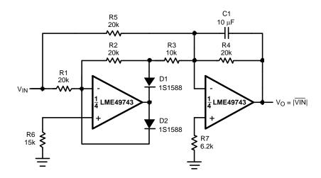
Figure 38. AC-DC Converter
