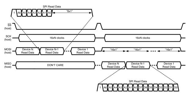
Figure 8. SPI Daisy-Chain Read
