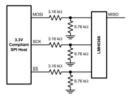
Figure 12. 3.3V SPI Interfacing
