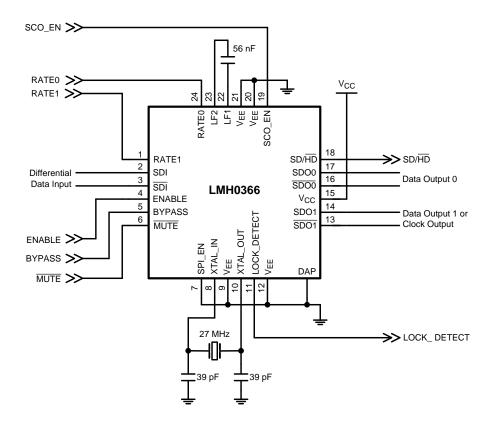
Figure 11. Application Circuit (Pin Mode)
