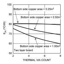
Figure 24. θ<sub>JA</sub> vs Thermal Via Count for the SO PowerPad Package on 2–Layer PCB with Copper Area on Bottom-Side
