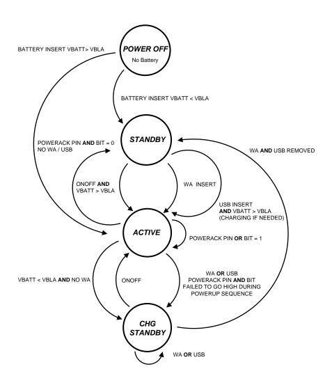
Figure 64. Operating Mode State Diagram
