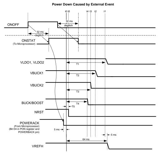
Figure 67. Power-Down Event Caused by External Event
