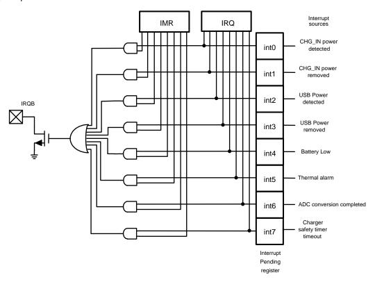
Figure 61. Interrupt Request Setting
