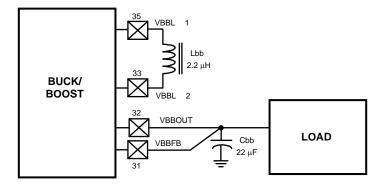
Figure 51. Schematic Section for Buck-Boost Operation
