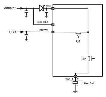
Figure 54. Switches for USB Charging Path
