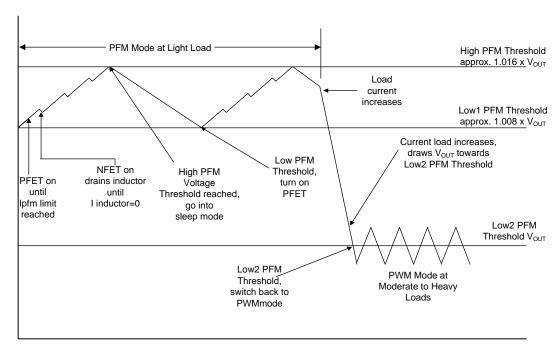
Figure 50. Operation in PFM Mode and Transfer to PWM Mode
