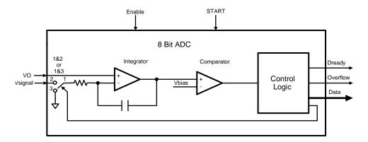
Figure 57. Simplified ADC Block Diagram
