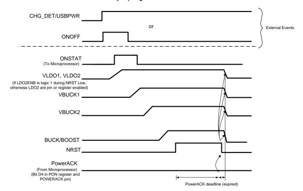
Figure 68. Power Down Caused by Expiring PowerACK Deadline
