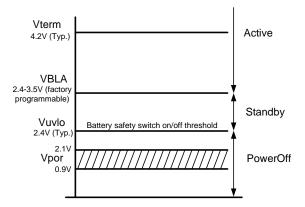
Figure 65. Voltage Threshold Levels
