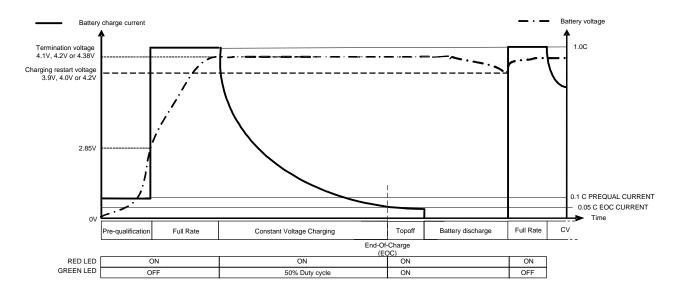
Figure 55. Charge Cycle Complete
