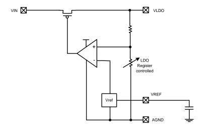
Figure 52. LDO Architecture Diagram
