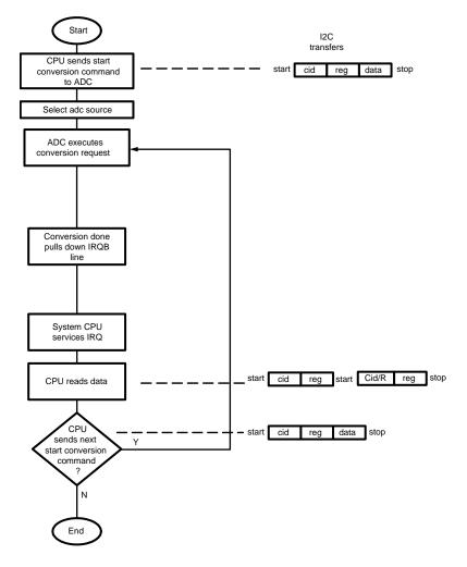
Figure 60. Data Measurement and Acquisition Sequence
