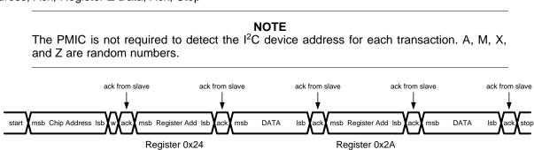
Figure 74. Example Multi-Byte Command Sequencing
