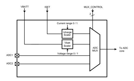
Figure 59. ADC Analog Front-End Block Diagram
