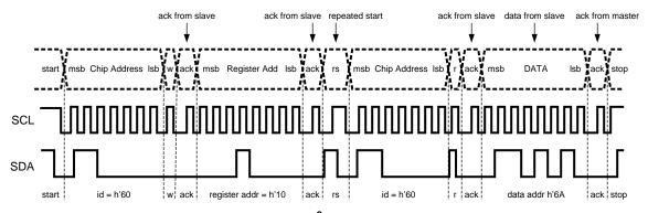
Figure 73. I<sup>2</sup>C Read Cycle
