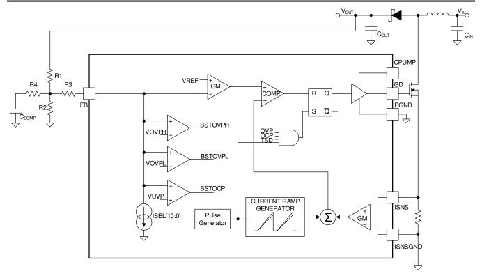
Figure 7-7. External Compensation Network
