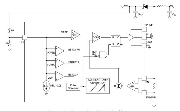
Figure 7-5. Two-Resistor FB Divider Circuit
