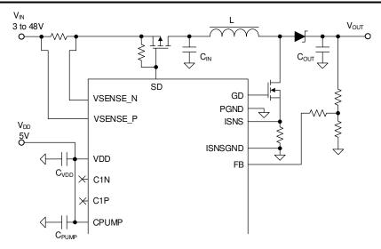
Figure 7-2. Charge Pump Disabled Circuit
