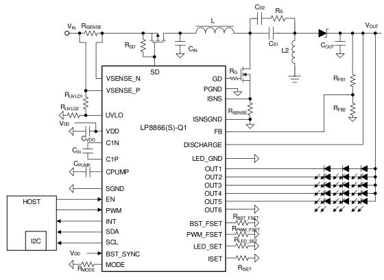
Figure 8-6. SEPIC Mode with Three LEDs in Series
