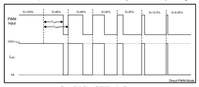
Figure 7-12. Direct PWM Dimming Diagram
