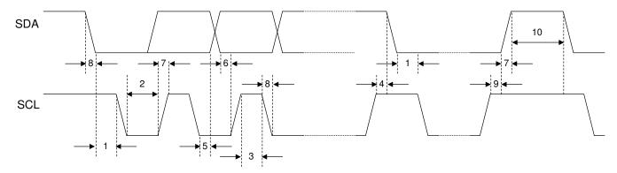
Figure 6-1. I2C Timing Diagram
