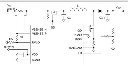
Figure 7-16. V<sub>IN</sub> UVLO Setting Circuit
