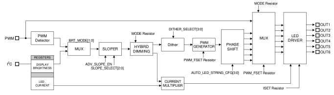
Figure 7-9. LP8866S-Q1 Brightness Path Diagram
