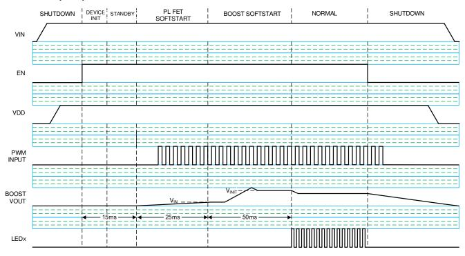
Figure 7-20. Start-Up Sequence Diagram
