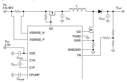
Figure 7-1. Charge Pump Enabled Circuit
