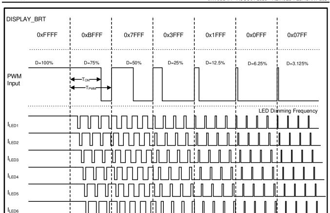
Figure 7-10. Phase-Shift Dimming Diagram
