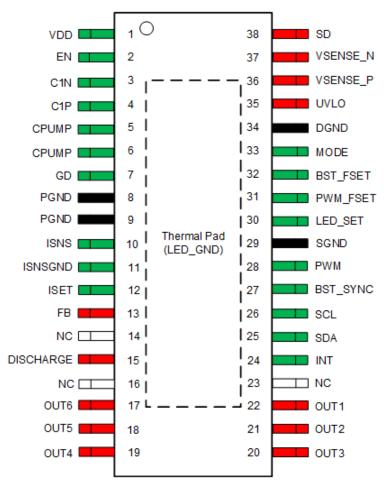
Figure 5-1. DCP Package 38-Pin HTSSOP Top View
