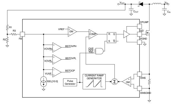
Figure 7-6. Three-Resistor FB Divider Circuit
