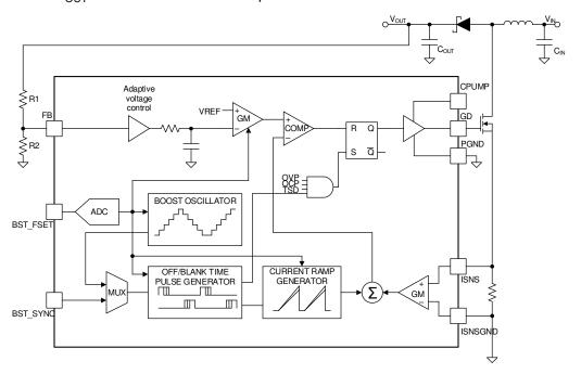
Figure 7-3. Boost Controller Block Diagram
