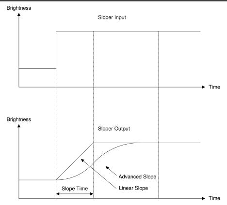
Figure 7-13. Brightness Sloper
