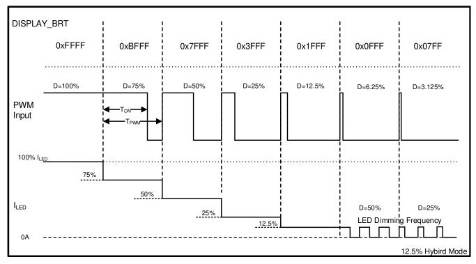
Figure 7-11. Hybrid Dimming Diagram
