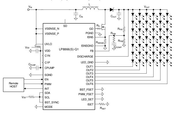
Figure 8-5. Minimal Solution/Minimum Components Application
