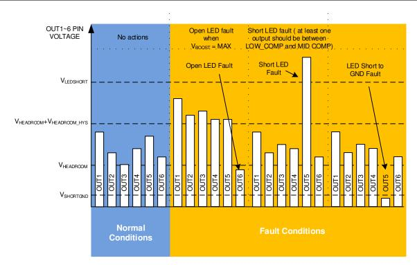
Figure 7-18. LED Open and Short Detection Logic
