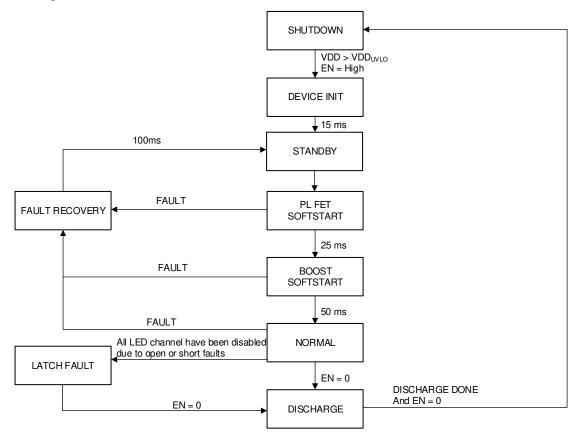
Figure 7-19. State Machine Diagram
