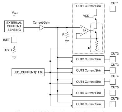
Figure 7-8. LED Driver Current Setting Circuit
