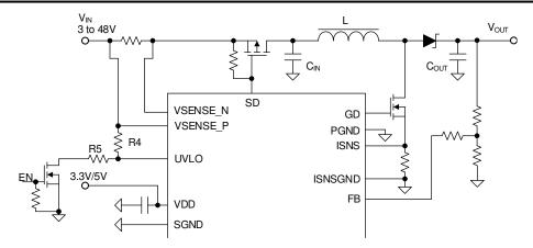
Figure 7-17. VIN UVLO Setting Circuit Without Current Leakage Path
