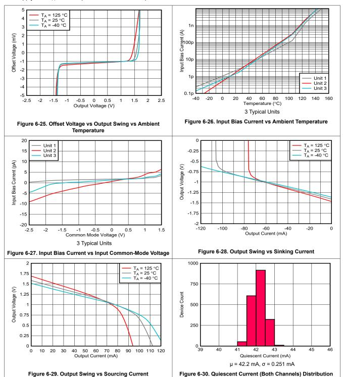
$V_{S+}$  = +2.5 V,  $V_{S-}$  = -2.5 V,  $R_L$  = 200  $\Omega$ ,  $C_{IN}$  = 4 pF, output load is referenced to mid-supply, input common-mode biased at mid-supply, and  $T_A \cong$  +25°C (unless otherwise noted)
