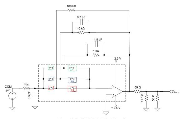
Figure 9-1. OPA3S2859 Test Circuit
