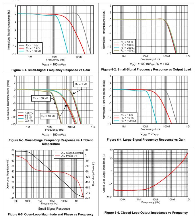
$V_{S+}$  = +2.5 V,  $V_{S-}$  = -2.5 V,  $R_L$  = 200  $\Omega$ ,  $C_{IN}$  = 4 pF, output load is referenced to mid-supply, input common-mode biased at mid-supply, and  $T_A \cong +25^{\circ}C$  (unless otherwise noted)
