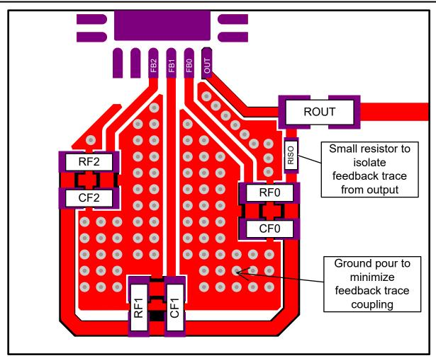
Figure 11-2. Feedback Network Layout Recommendations
