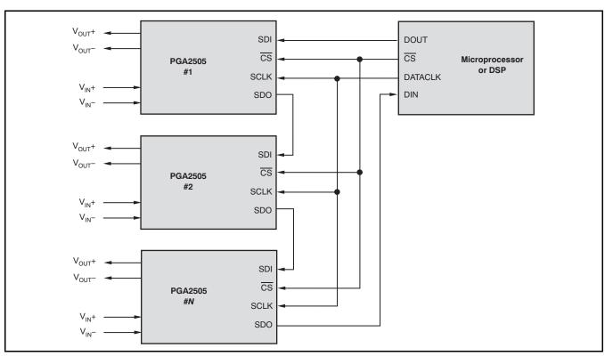
Figure 11. Daisy-Chain Configuration for Multiple PGA2505 Preamplifiers
