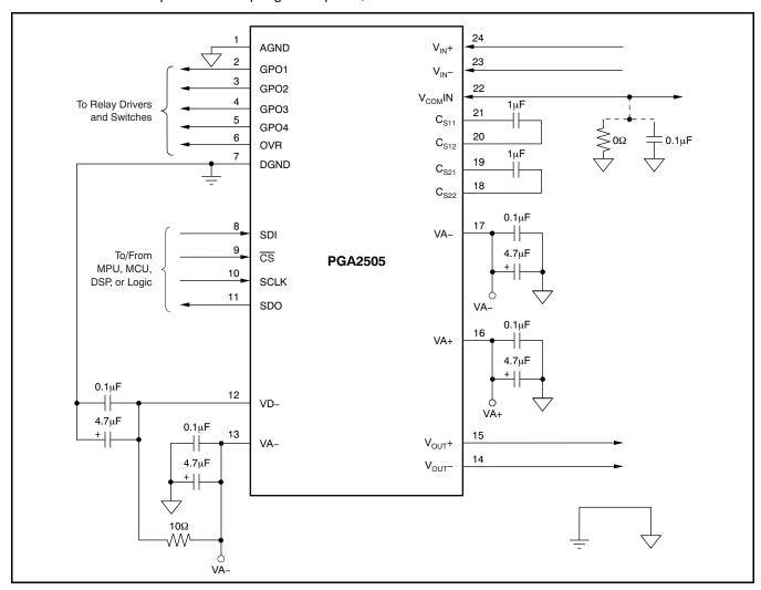
Figure 13. Basic Circuit Configuration for the PGA2505
