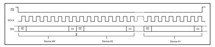
Figure 12. Serial Port Operation for Daisy-Chain Operation
