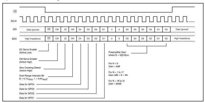
Figure 10. Serial Port Protocol
