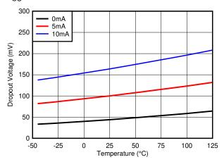
Figure 11-1. Dropout Voltage vs Temperature
