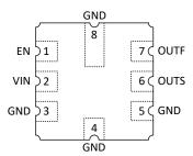
Figure 6-1. FKH Package 8-Pin LCCC Top View
