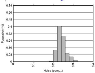
Figure 8-10. 0.1-Hz to 10-Hz Voltage Noise Distribution
