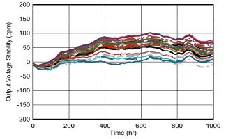
Figure 7-26. Long-Term Stability VSSOP package
