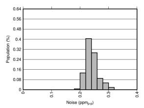
0.1-Hz to 10-Hz Voltage Noise Distribution
