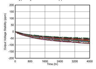
Figure 8-4. Long Term Stability LCCC -4000 hours (V<sub>OUT</sub>)
