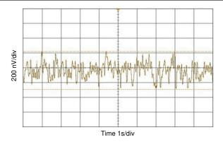
Figure 8-11. 0.1-Hz to 10-Hz Voltage Noise
