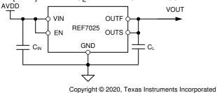
Figure 9-1. Basic Connections
