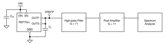
Figure 8-12. Broadband Noise Test Setup
