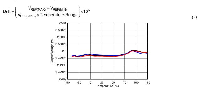
Figure 8-14. Output Voltage Vs Free-Air Temperature
