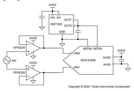
Figure 10-1. Basic Reference Connection
