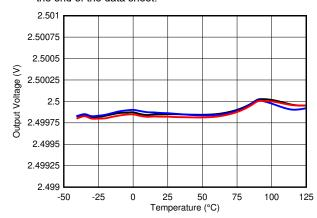
Output Voltage Vs Free-Air-Temperature
