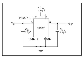
FIGURE 3. Typical Operating Circuit.
