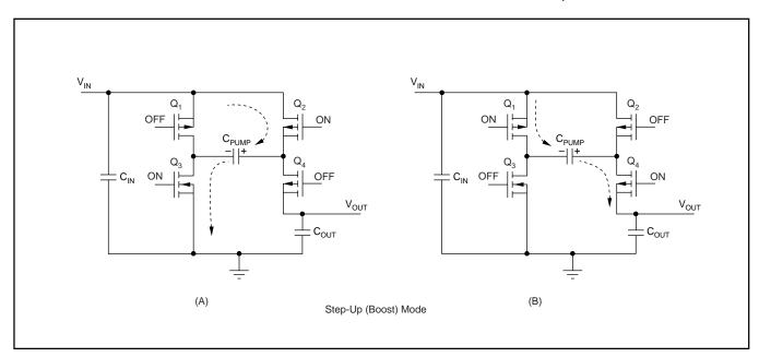
FIGURE 2. Simplified Schematic of the REG711 Operating in the Step-Up or Boost Mode.
