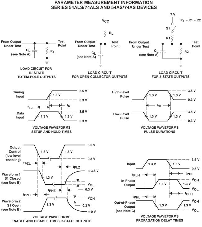
NOTES: A. CL includes probe and jig capacitance.
