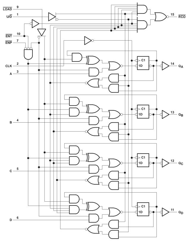
logic diagram (positive logic)
