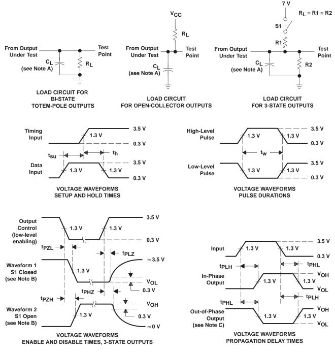
NOTES: A. C<sub>L</sub> includes probe and jig capacitance.
