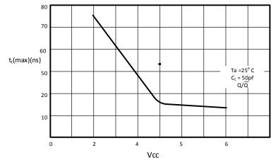
Figure 9-1. Maximum Transition Time vs  $\ensuremath{V_{CC}}$
