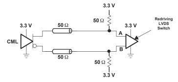
Figure 9-2. Current-Mode Logic (CML)
