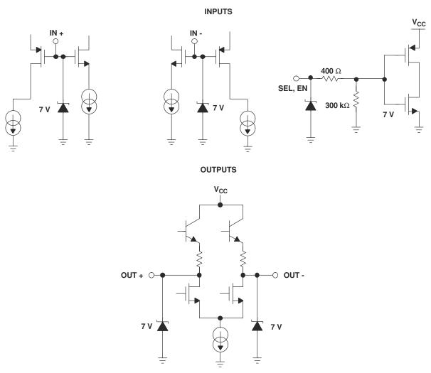
Figure 7-1. Equivalent Input and Output Schematic Diagrams
