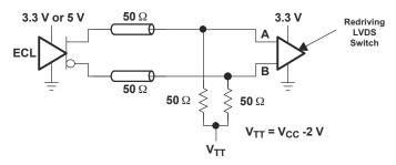
Figure 9-1. Low-Voltage Positive Emitter-Coupled Logic (LVPECL)
