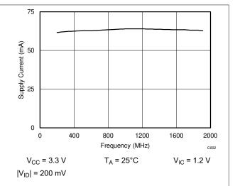
Figure 6-2. Supply Current vs Frequency
