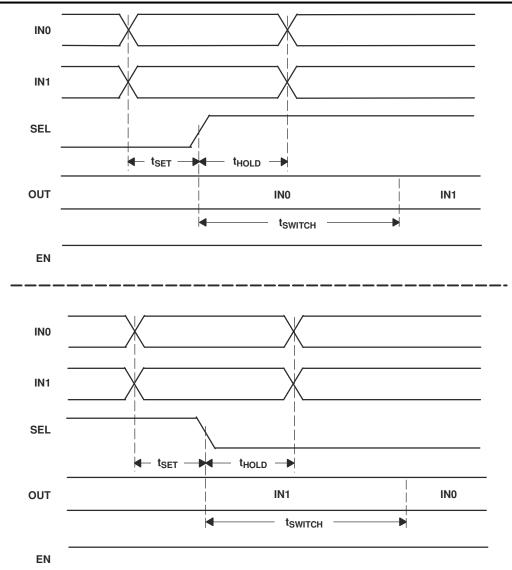
$t_{\mathsf{SET}}$  and  $t_{\mathsf{HOLD}}$  times specify that data must be in a stable state before and after mux control switches.
