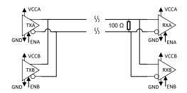
Figure 9-5. LVDS Cold sparing example
