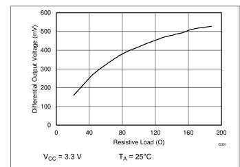
Figure 6-1. Differential Output Voltage vs Resistive Load
