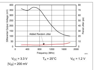
Figure 6-11. Peak-To-Peak Jitter vs Data Rate
