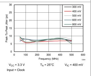
Figure 6-4. Peak-To-Peak Jitter vs Frequency
