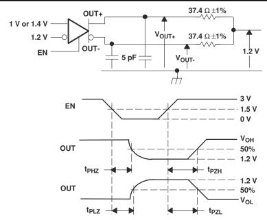
All input pulses are supplied by a generator having the following characteristics:  $t_r$  or  $t_f \le 1$  ns, pulse-repetition rate (PRR) = 0.5 Mpps, pulse width =  $500 \pm 10$  ns.  $C_L$  includes instrumentation and fixture capacitance within 0,06 mm of the D.U.T.
