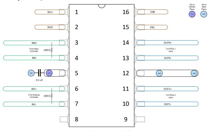
Figure 11-1. Layout Example with LVDS input signals
