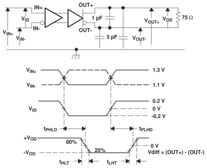
All input pulses are supplied by a generator having the following characteristics:  $t_f$  or  $t_f \le .25$  ns, pulse-repetition rate (PRR) = 0.5 Mpps, pulse width =  $500 \pm 10$  ns.  $C_L$  includes instrumentation and fixture capacitance within 0,06 mm of the D.U.T.
