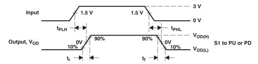
Figure 3. Driver Delay and Transition Time Test Waveforms
