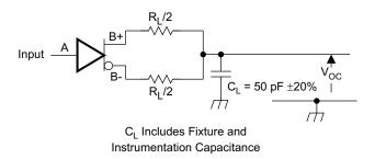
Figure 1. Driver Test Circuit, RS-422 and RS-485 Loading
