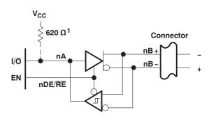
(b) ACTIVE-LOW BIDIRECTIONAL I/O WITH SEPARATE ENABLE
