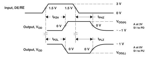
Figure 7. Driver Enable Time Waveforms
