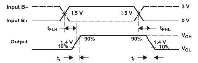
Figure 5. Receiver Delay and Transition Time Waveforms
