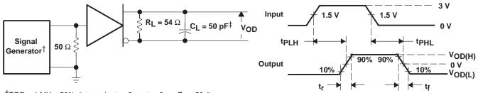
†PRR = 1 MHz, 50% duty cycle,  $t_{\rm f}$  < 6 ns,  $t_{\rm f}$  < 6 ns,  $Z_{\rm O}$  = 50  $\Omega$  ‡Includes probe and jig capacitance
