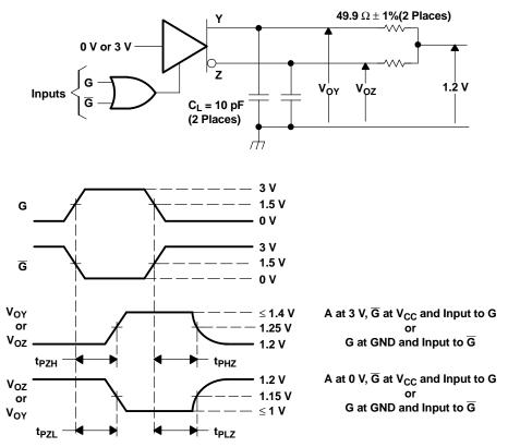
NOTE: All input pulses are supplied by a generator having the following characteristics:  $t_r$  or  $t_f \le 1$  ns, pulse repetition rate (PRR) = 0.5 Mpps, pulse width = 500 ±10 ns.  $C_L$  includes instrumentation and fixture capacitance within 0,06 mm of the DUT.
