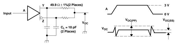
NOTE: All input pulses are supplied by a generator having the following characteristics:  $t_r$  or  $t_f \le 1$  ns, pulse repetition rate (PRR) = 0.5 Mpps, pulse width = 500 ±10 ns.  $C_L$  includes instrumentation and fixture capacitance within 0,06 mm of the DUT. The measurement of  $V_{OC(PP)}$  is made on test equipment with a -3 dB bandwidth of at least 300 MHz.
