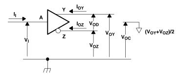
Figure 1. Driver Voltage and Current Definitions
