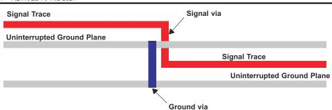
Figure 12-7. Ground Via Location (Side View)
