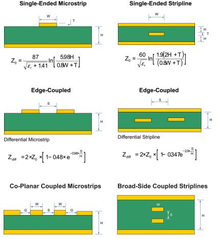
Figure 10-4. Controlled-Impedance Transmission Lines
