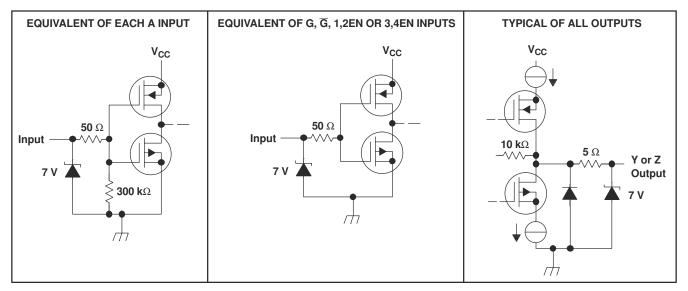
Figure 9-1. Equivalent Input and Output Schematic Diagrams
