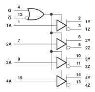
SN65LVDS3487 logic diagram (positive logic)
