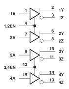
SN65LVDS9638 logic diagram (positive logic)
