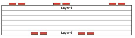
Figure 12-6. Staggered Trace Layout
