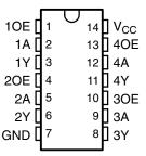
To ensure the high-impedance state during power up or power down, OE should be tied to GND through a pulldown resistor; the minimum value of the resistor is determined by the current-sourcing capability of the driver.
