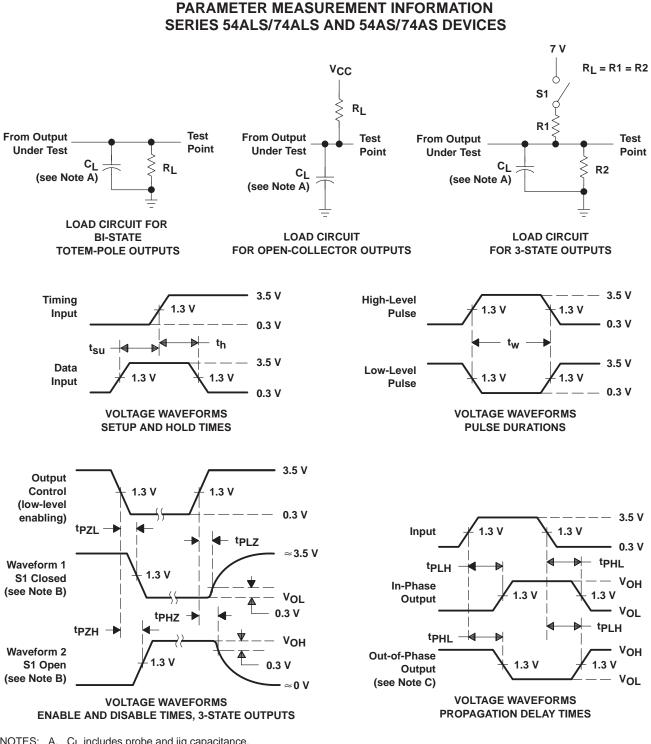
NOTES: A. CL includes probe and jig capacitance.
