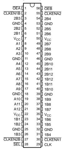
To ensure the high-impedance state during power up or power down, a clock pulse should be applied as soon as possible, and  $\overline{OE}$  should be tied to  $V_{CC}$  through a pullup resistor; the minimum value of the resistor is determined by the current-sinking capability of the driver. Due to  $\overline{OE}$  being routed through a register, the active state of the outputs cannot be determined prior to the arrival of the first clock pulse.
