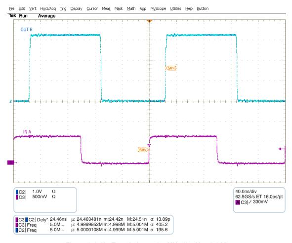
Figure 9-2. Up Translation at 2.5 MHz (0.7 V to 3.3 V)
