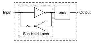
Figure 8-2. Simplified Schematic for Device With Bus-Hold Data Inputs
