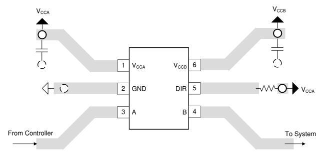
Figure 11-1. PCB Layout Example
