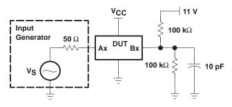
Figure 1. Device Test Setup
