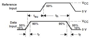
Figure 7-3. Voltage Waveforms
