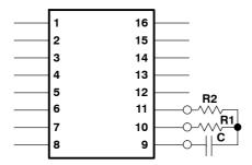
To determine the values of capacitance and resistance necessary to obtain a specific oscillator frequency (f), use this formula:
