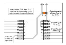
Figure 11-1. Example layout for the SN74HC7032
