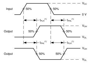
(1) The greater between t<sub>PLH</sub> and t<sub>PHL</sub> is the same as t<sub>pd</sub>. Figure 7-4. Voltage Waveforms Propagation Delays
