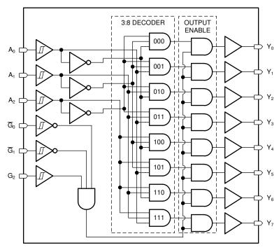
Figure 8-1. Logic Diagram (Positive Logic) for SN74HCS238
