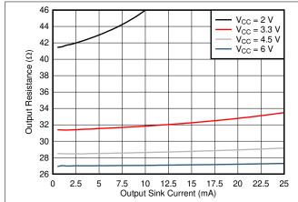
Figure 6-1. Output driver resistance in LOW state.
