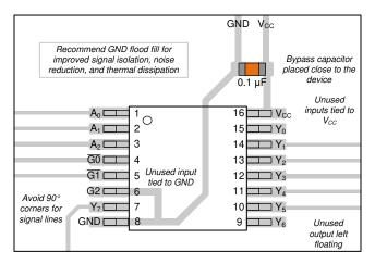
Figure 11-1. Example layout for the SN74HCS238.
