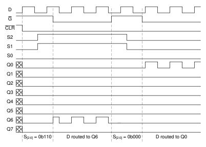
Figure 9-2. Application timing diagram
