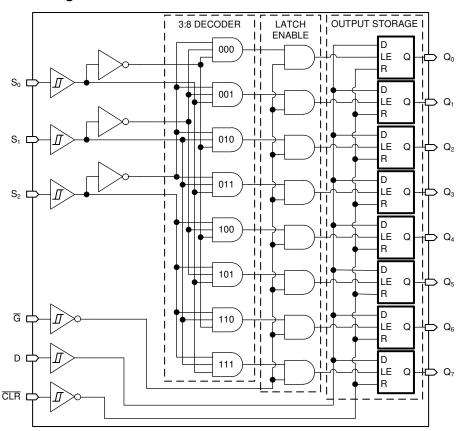
Figure 8-1. Logic Diagram (Positive Logic) for SN74HCS259
