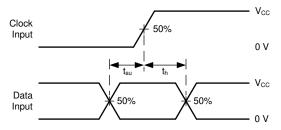
Figure 7-3. Voltage Waveforms, Setup and Hold Times
