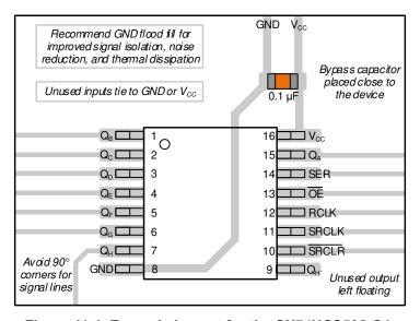
Figure 11-1. Example Layout for the SN74HCS595-Q1.
