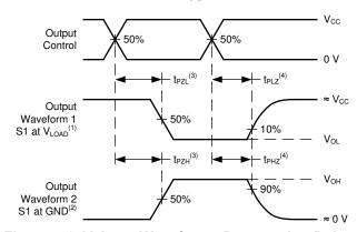
Figure 7-6. Voltage Waveforms Propagation Delays
