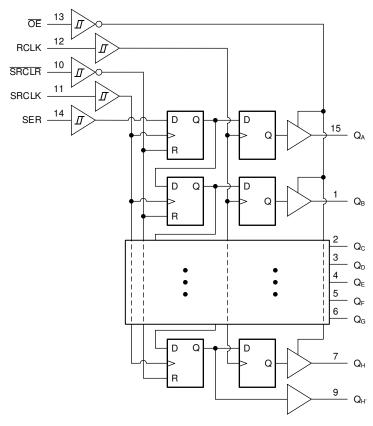
Figure 8-1. Logic Diagram (Positive Logic) for the SN74HCS595-Q1
