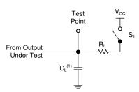
(1) C<sub>L</sub> includes probe and test-fixture capacitance.
