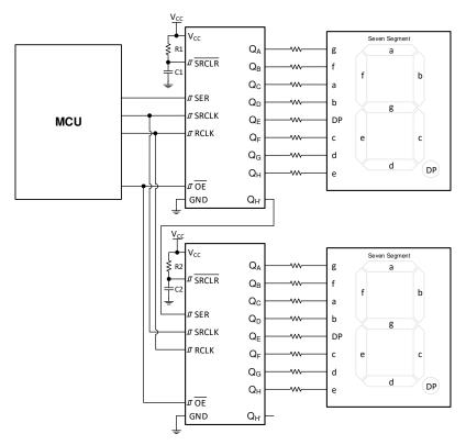
Figure 9-1. Typical application block diagram
