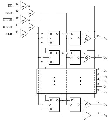
Figure 8-1. Logic Diagram (Positive Logic) for SN74HCS596
