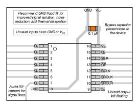
Figure 11-1. Example layout for the SN74HCS596.
