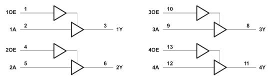
Pin numbers shown are for the D, DB, DGV, J, N, NS, PW, and W packages.
