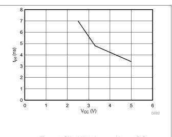
Figure 2. SN74LV126A  $t_{PD}\ vs\ V_{CC}$  at 25°C
