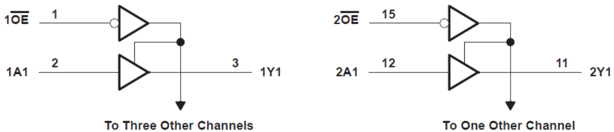
Figure 8-1. Logic Diagram (Positive Logic)
