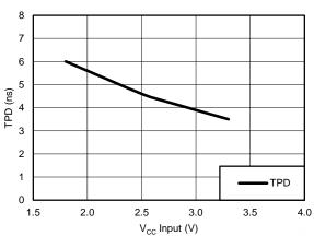
Figure 1. TPD vs  $V_{CC}$  ( $T_A = 25^{\circ}C$ )
