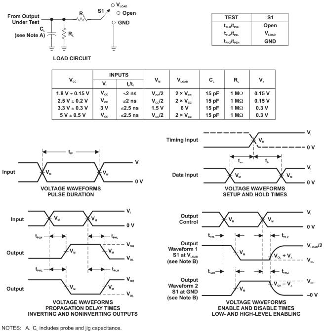
B. Waveform 1 is for an output with internal conditions such that the output is low, except when disabled by the output control. Waveform 2 is for an output with internal conditions such that the output is high, except when disabled by the output control. C. All input pulses are supplied by generators having the following characteristics: PRR  $\leq$  10 MHz, Z<sub>0</sub> = 50  $\Omega$ .
