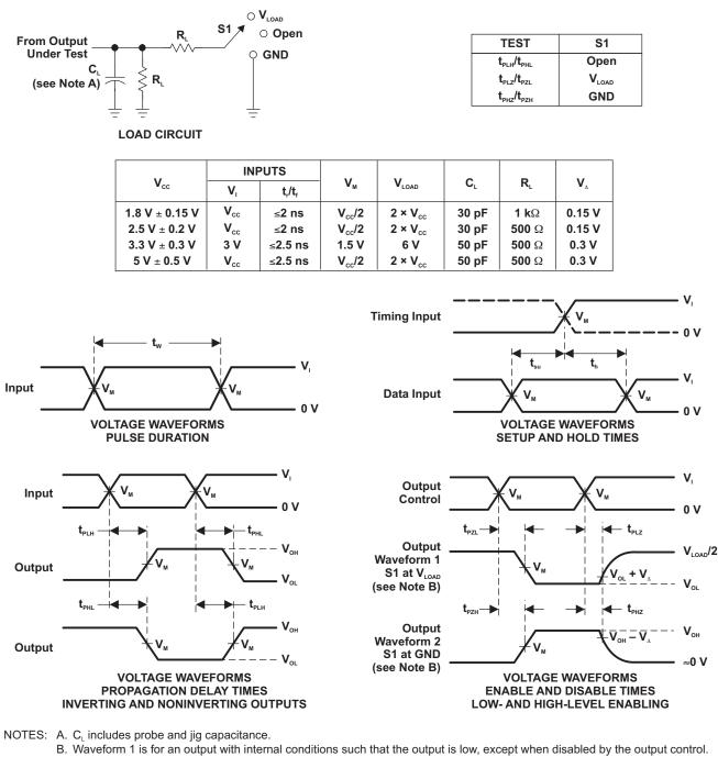
Waveform 2 is for an output with internal conditions such that the output is high, except when disabled by the output control. C. All input pulses are supplied by generators having the following characteristics: PRR  $\leq$  10 MHz, Z<sub>o</sub> = 50  $\Omega$ .
