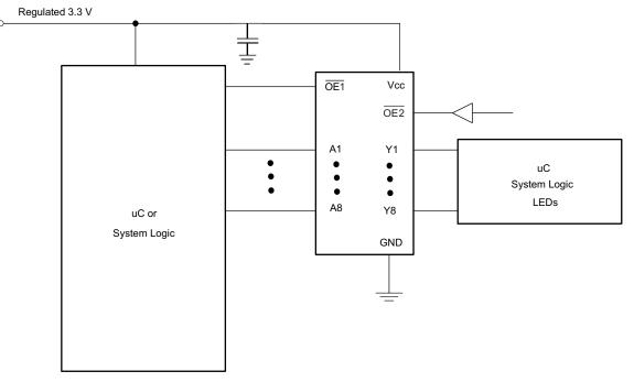
Figure 4. Typical Application Diagram
