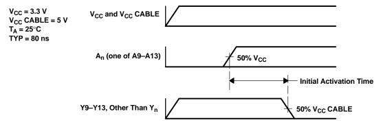
One of pins A9-A13 is switched as shown above, and the other four inputs are forced at low state.
