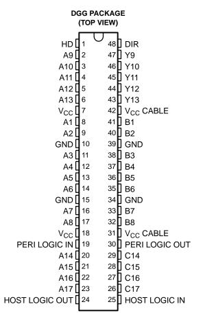
This device has eight bidirectional bits; data can flow in the A-to-B direction when the direction-control (DIR) input is high and in the B-to-A direction when DIR is low. This device also has five drivers that drive the cable side and four receivers. The SN74LVCZ161284A has one receiver dedicated to the HOST LOGIC line and a driver to drive the PERI LOGIC line.
