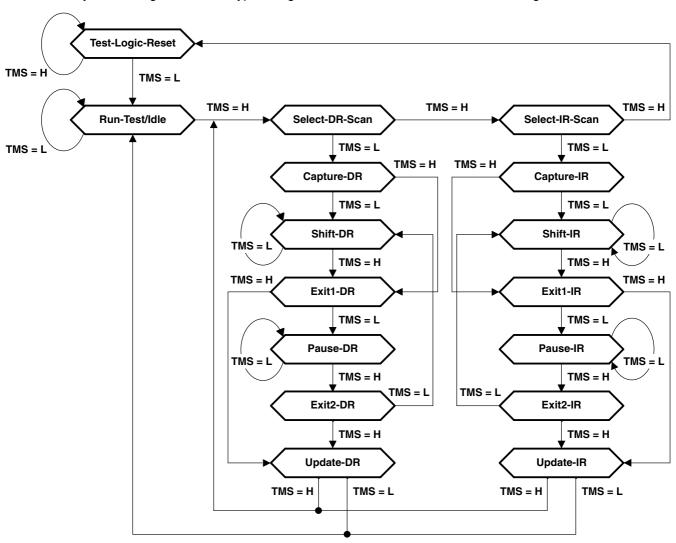
Figure 1. TAP-Controller State Diagram
