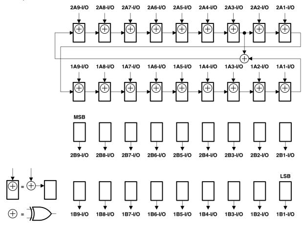
Figure 11. 18-Bit PSA/COUNT Configuration  $(1\overline{OEAB} = 2\overline{OEAB} = 0, 1\overline{OEBA} = 2\overline{OEBA} = 1)$
