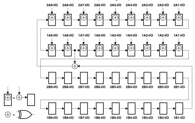
Figure 7. 36-Bit PSA Configuration (1OEAB = 2OEAB = 0, 1OEBA = 2OEBA = 1)
