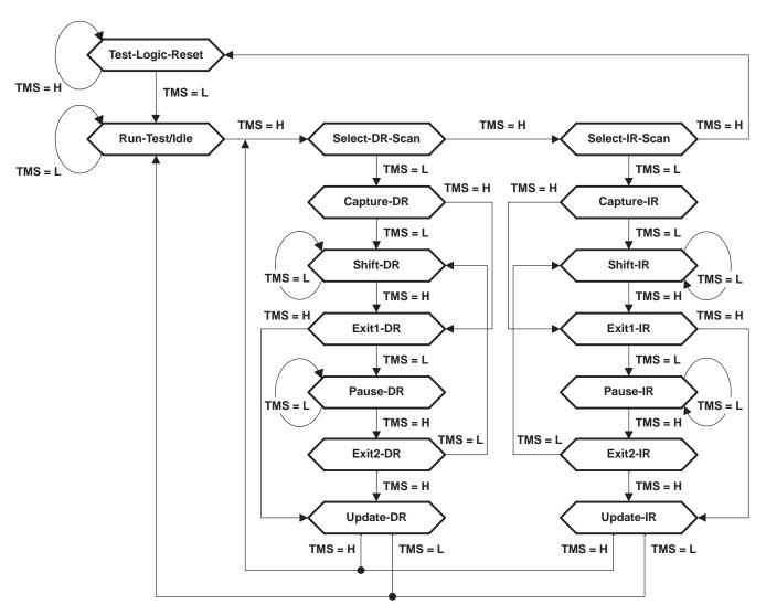
Figure 1. TAP-Controller State Diagram
