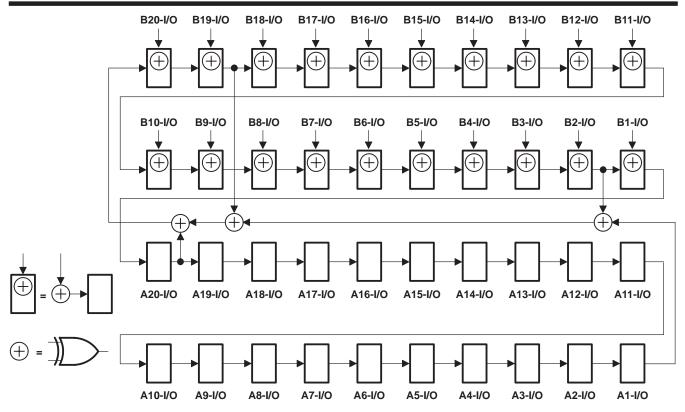
Figure 8. 40-Bit PSA Configuration ( $\overline{OEAB} = 1$ ,  $\overline{OEBA} = 0$ )
