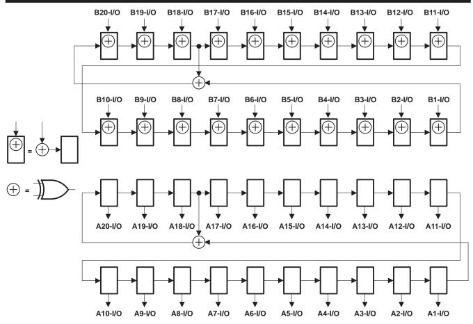
Figure 10. 20-Bit PSA/PRPG Configuration (OEAB = 1, OEBA = 0)
