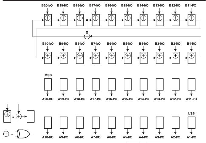
Figure 12. 20-Bit PSA/COUNT Configuration (OEAB = 1, OEBA = 0)
