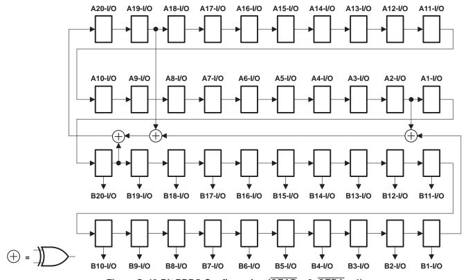
Figure 5. 40-Bit PRPG Configuration ( $\overline{OEAB} = 0$ ,  $\overline{OEBA} = 1$ )
