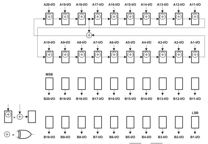
Figure 11. 20-Bit PSA/COUNT Configuration (OEAB = 0, OEBA = 1)
