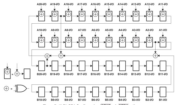
Figure 7. 40-Bit PSA Configuration ( $\overline{OEAB} = 0$ ,  $\overline{OEBA} = 1$ )
