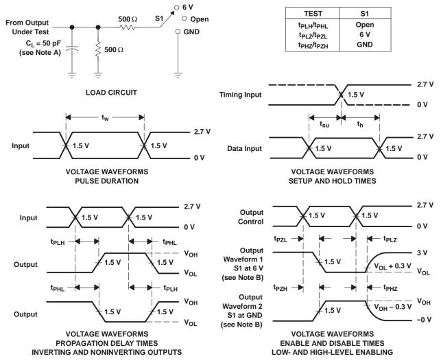
NOTES: A. CL includes probe and jig capacitance.
