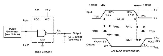
NOTES: A. The pulse generator has the following characteristics: PRR = 1 MHz,  $Z_O \approx 50~\Omega$ .
