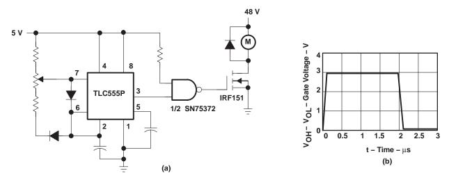
Figure 14. Power MOSFET Drive Using SN75372
