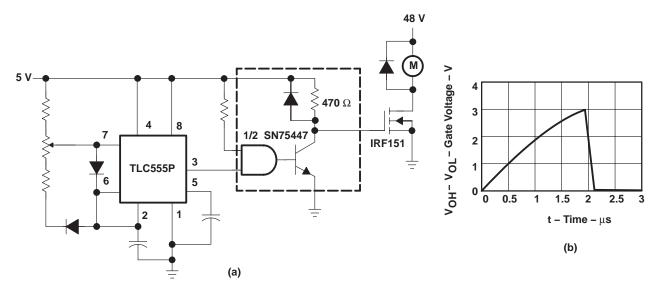
Figure 13. Power MOSFET Drive Using SN75447
