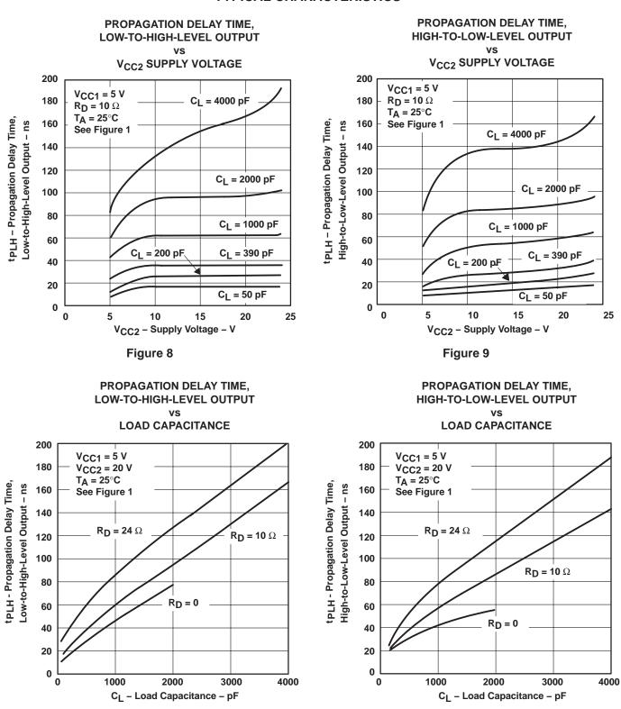
NOTE: For  $R_D = 0$ , operation with  $C_L > 2000 \ pF$  violates absolute maximum current rating.
