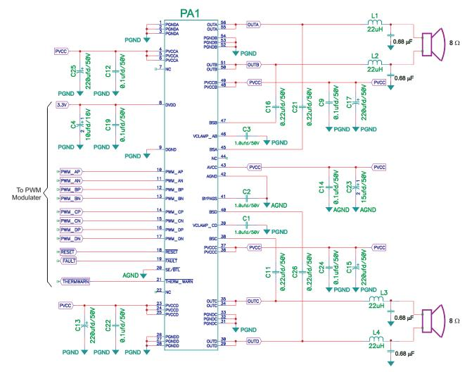
Figure 1. Bridge Tied Load (BTL) Application Schematic
