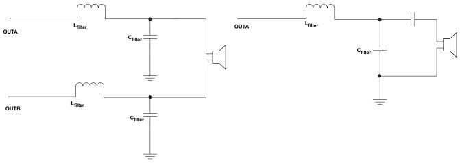
Figure 17. BTL Filter Configuration
