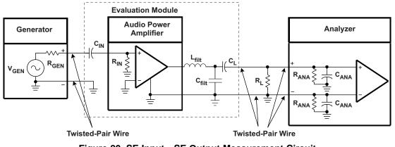
Figure 20. SE Input—SE Output Measurement Circuit
