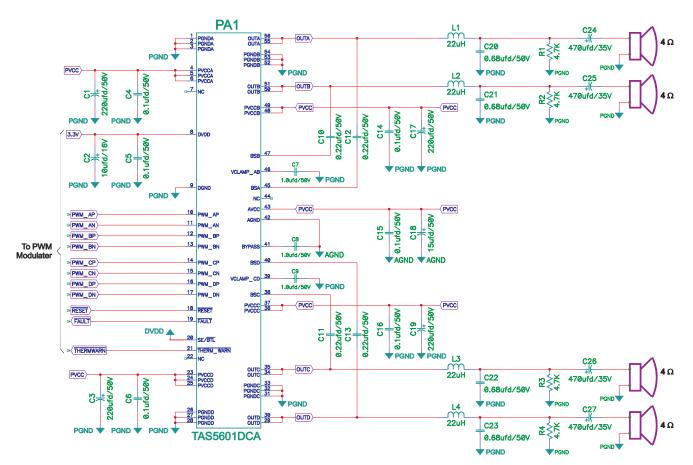
Figure 2. Single Ended (SE) Application Schematic
