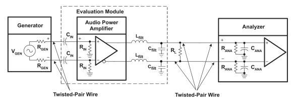
Figure 21. Differential Input, BTL Output Measurement Circuit
