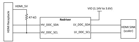
Figure 8-8. Sink Application: DDC Buffer Enabled
