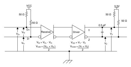
Figure 7-2. TMDS Main Link Test Circuit
