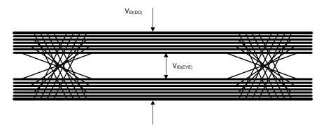
Figure 7-10.  $V_{ID(DC)}$  and  $V_{ID(EYE)}$
