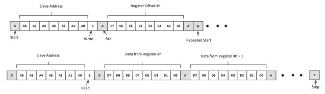
Figure 8-13. I2C Read with repeated Start
