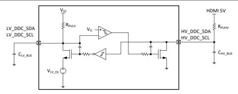
Figure 8-4. DDC Buffer Block Diagram
