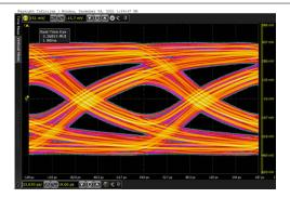
Figure 9-8. 5.94 Gbps Input Eye at TTP2 After Pre-Channel
