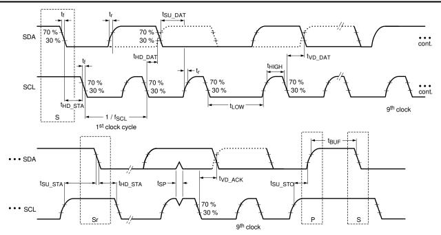
Figure 7-9. I<sup>2</sup>C SCL and SDA Timing
