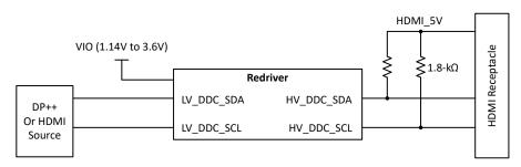
Figure 8-5. Source Application: DDC Buffer Enabled
