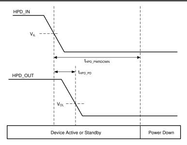
Figure 7-7. HPD Logic Shutdown and Propagation Timing
