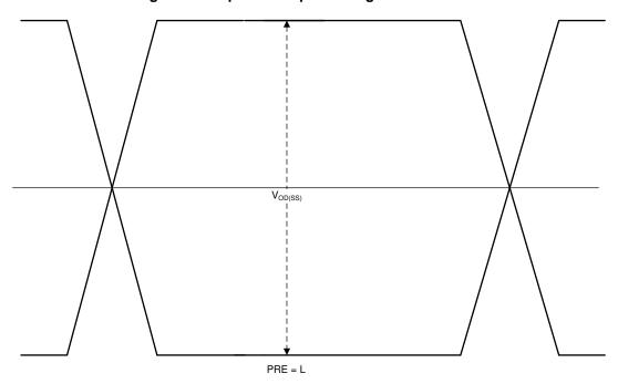
Figure 7-4. Output Differential Waveform
