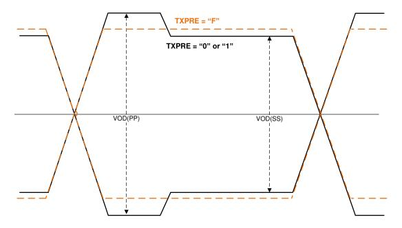
Figure 7-5. Output Differential Waveform with De-Emphasis
