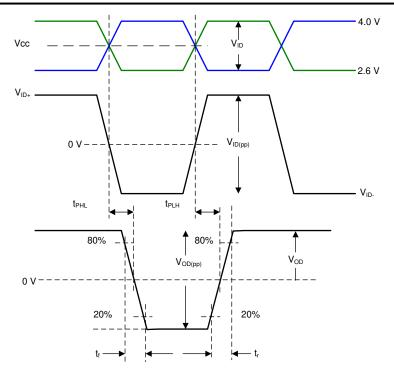
Figure 7-3. Input or Output Timing Measurements
