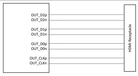
Figure 8-2. DC-Coupled TX in HDMI Source Application (AC EN = Low). External ESD Not Shown.
