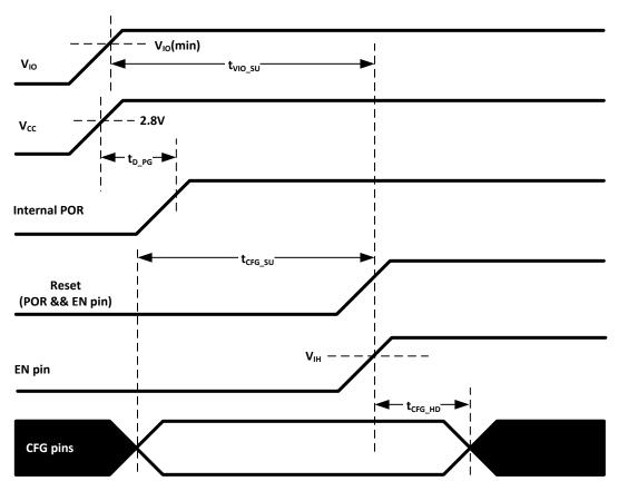
Figure 7-1. Power-On Timing Requirements
