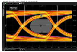
Figure 9-6. 2.97 Gbps Input Eye at TTP2 After Pre-Channel
