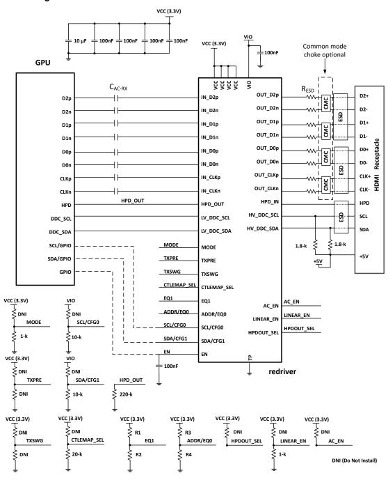
Figure 9-2. TDP0604 in Source Application Schematics
