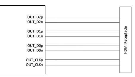
Figure 8-2. DC-Coupled TX in HDMI Source Application (AC\_EN = Low). External ESD is Not Shown.
