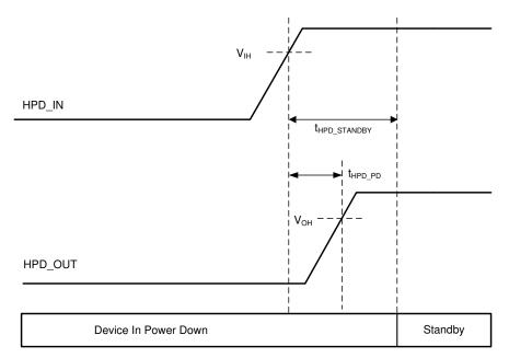
Figure 7-8. HPD Logic Standby and Propagation Timing
