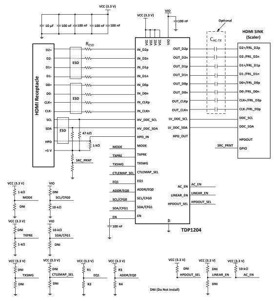
Figure 9-10. TDP1204 in Sink Application Schematics
