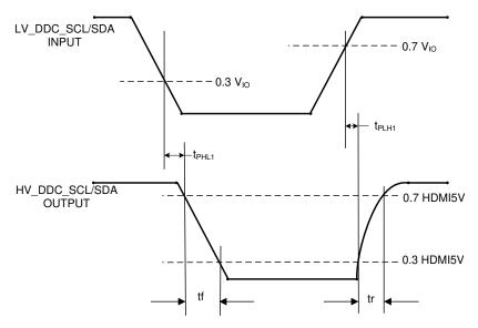
Figure 7-10. DDC Propagation Delay – Source to Sink
