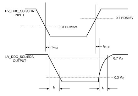
Figure 7-11. DDC Propagation Delay – Sink to Source
