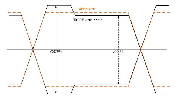
Figure 7-5. Output Differential Waveform with De-Emphasis
