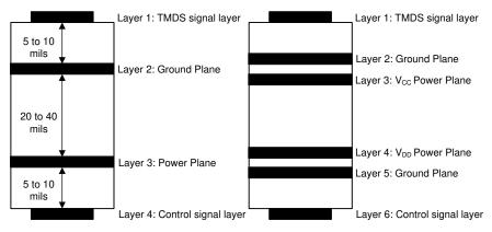
Figure 11-1. Recommended 4 or 6-Layer PCB Stack
