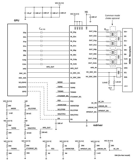
Figure 9-2. TDP1204 in Source Application Schematics
