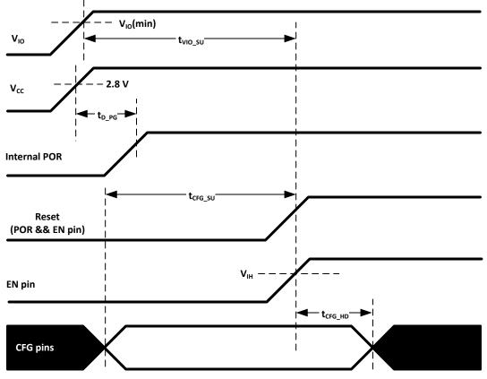
Figure 7-1. Power-On Timing Requirements
