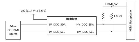
Figure 8-5. Source Application: DDC Buffer Enabled
