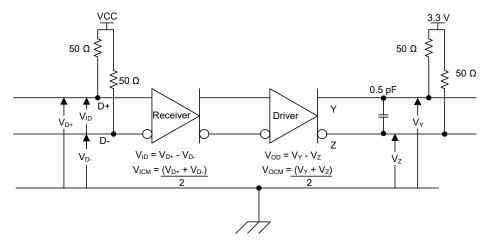
Figure 7-2. TMDS Main Link Test Circuit
