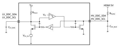
Figure 8-4. DDC Buffer Block Diagram
