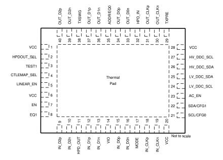
Figure 5-1. RNQ Package 40-Pin WQFN (Top View)
