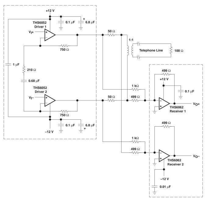
Figure 1. THS6052 ADSL Application With 1:1 Transformer Ratio
