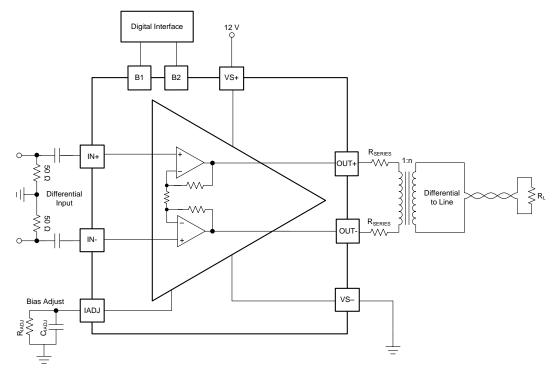
Figure 41. G.Fast, 212-MHz Driving Mode Example Circuit
