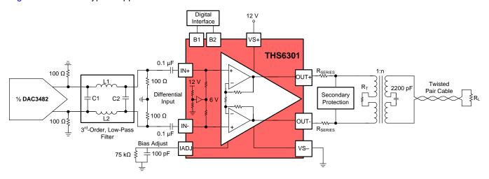
Figure 42. Typical G.FAST Line Driver Configuration
