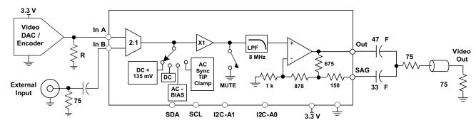
Figure 1. 3.3 V Single-Supply DC-Input/AC-Video Output System w/SAG Correction (1 of 3 Channels Shown)
