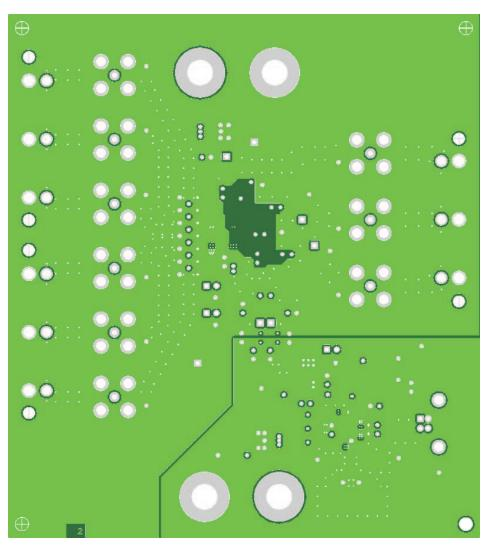
Figure 67. Layer Two - Ground Layer
