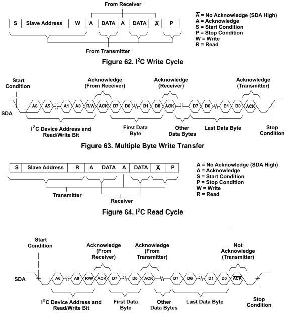
Figure 65. Multiple Byte Read Transfer
