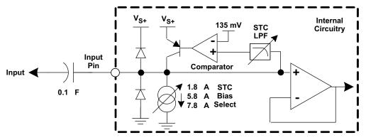
Figure 51. Equivalent AC Sync Tip Clamp Input Mode Circuit
