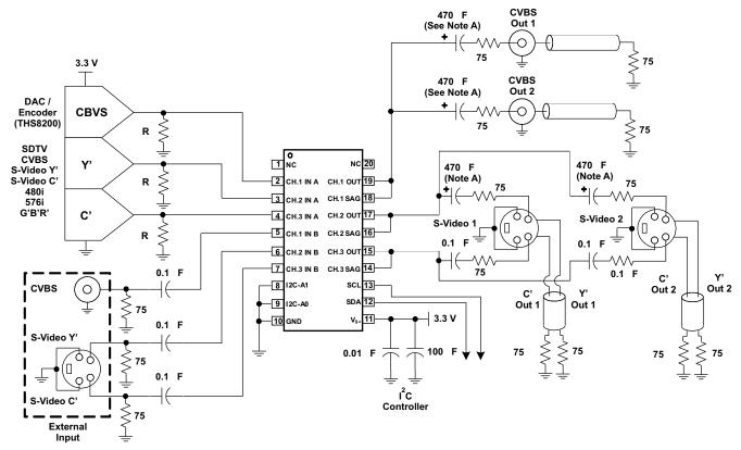
A. Due to the high frequency content of the video signal, it is recommended, but not required, to add a 0.01-µF capacitor in parallel with these large capacitors.
