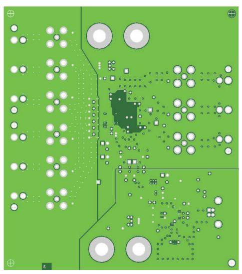
Figure 68. Layer Three - Power and Ground Layer
