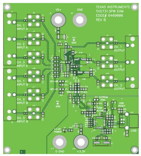
Figure 66. Top Layer - Signal Layer
