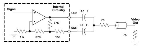
Figure 54. THS7313 Output Buffer Using SAG Corrected AC-Coupling
