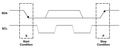
Figure 58. I<sup>2</sup>C Start and Stop Conditions
