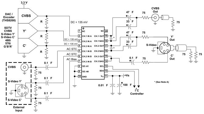
A. If the SAG correction capacitors are more than 15 mm from the THS7313, add a  $0.01\mu$ F capacitor as shown.
