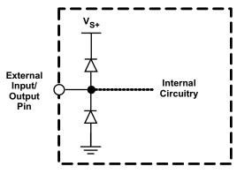
Figure 46. Internal ESD Protection
