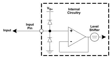
Figure 49. Equivalent DC + 135 mV Input Mode Circuit
