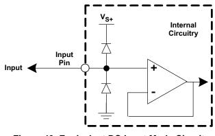
Figure 48. Equivalent DC Input Mode Circuit
