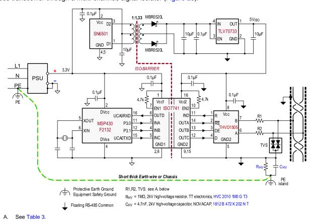
Figure 29. Isolated Bus Node With Transient Protection
