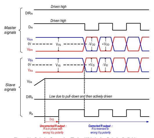
Figure 21. Polarity Correction Timing With Active Polarity Definition
