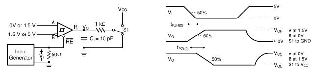
Figure 16. Measurement of Receiver Enable Times With Driver Disabled
