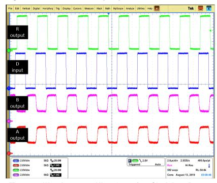
Figure 31. Waveforms at 1 Mbps Operation, Clock Data Pattern
