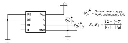
Figure 12. Measurement of Bus Impedance
