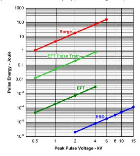
Figure 27. Comparison of Transient Energies
