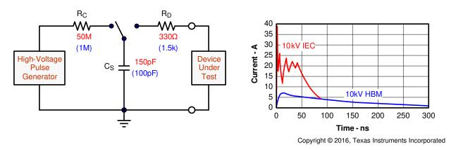
Figure 25. HBM and IEC ESD Models and Currents in Comparison (HBM Values in Parenthesis)
