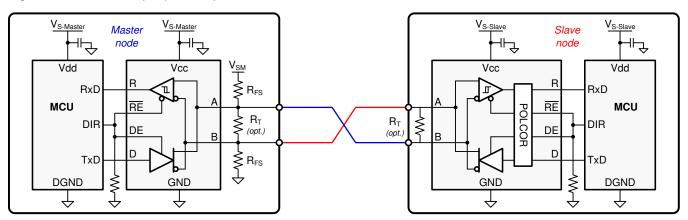
Figure 18. Passive Polarity Definition
