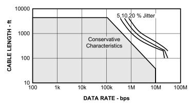
Figure 23. Cable Length vs Data Rate Characteristic
