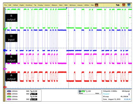
Figure 30. Waveforms at 1 Mbps Operation, PRBS7 Data Pattern
