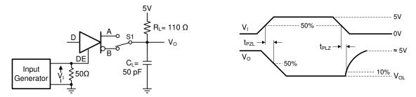
Figure 11. Measurement of Driver Enable and Disable Times With Active-Low Output and Pull-up Load
