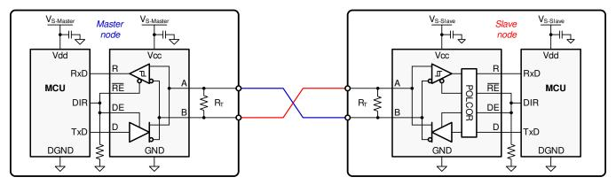
Figure 20. Active Polarity Definition
