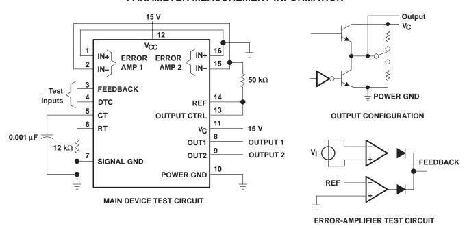
**Figure 1. Test Circuits**
