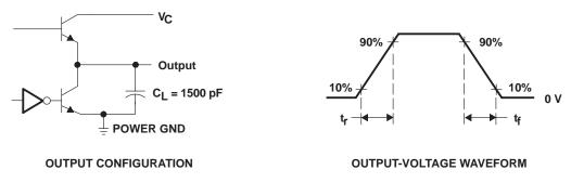
Figure 2. Switching Output Configuration and Voltage Waveform
